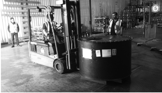
Figure 2. Polyethylene transport tank used for Mola mola : (1.4 m diam. \times 0.92 m high) with 750 L capacity. The tank flies completely sealed, (IATA LAR 60) with a small aeration unit mounted under the lid. The unit dissolves oxygen that was added previously into the water. The water level is approximately half of the height. Photo taken and permission granted by: João Correia, Flying Sharks.
